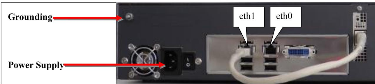
*Figure 1: Grounding Screw on XV3000 Rear Panel*
