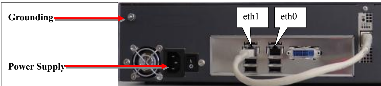
Figure 1: Grounding Screw on XV0500 Rear Panel
