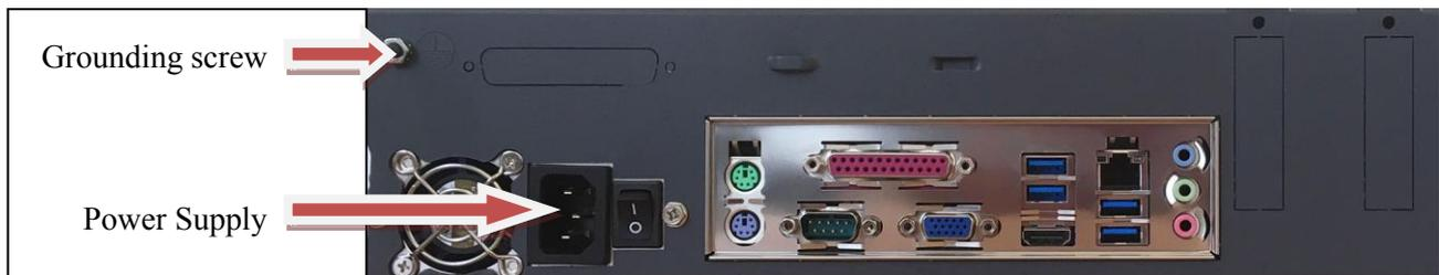
Figure 1: Grounding Screw on XR2000 Rear Panel
