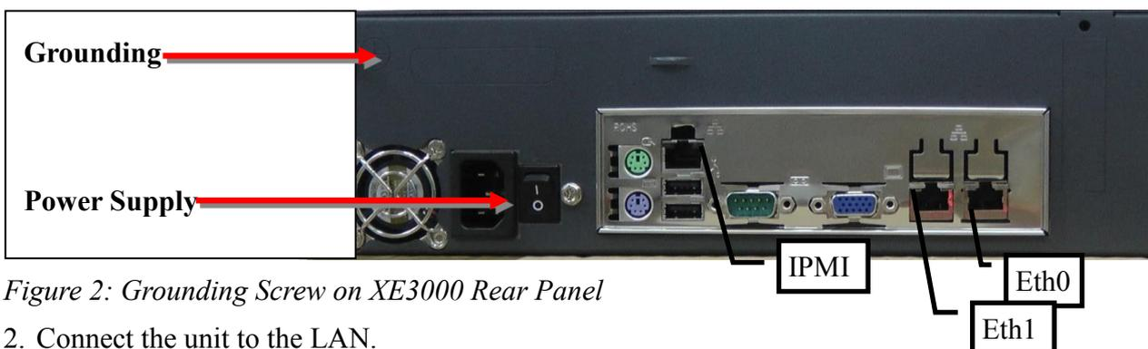
Figure 2: Grounding Screw on XE3000 Rear Panel
