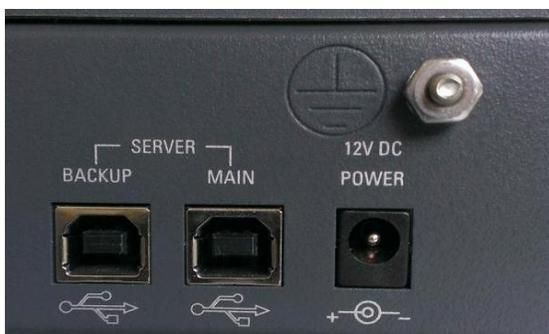
Once powered up, the Atribank will always use the “Main” USB interface, which must be connected to the preferred Master server. The “Backup” USB interface must be connected to the preferred Slave server.
