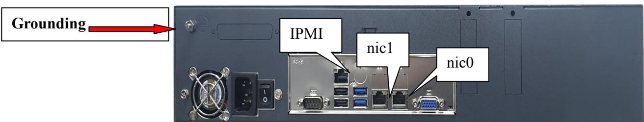
Figure 2: Detail of CXE3000 Rear Panel
