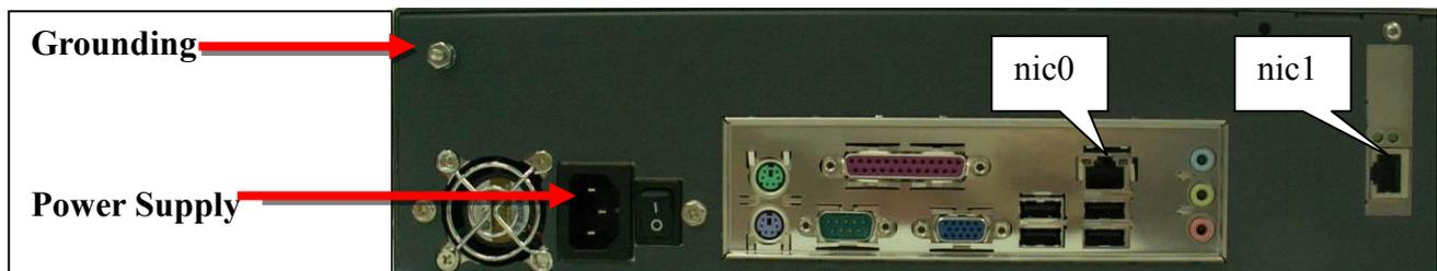
Figure 1: Detail of CXE2000 Rear Panel
