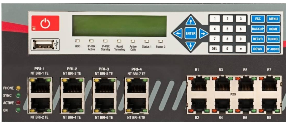
Fig. 3 – BRI/PRI Panel (allows up to additional 24 FXS ports)
