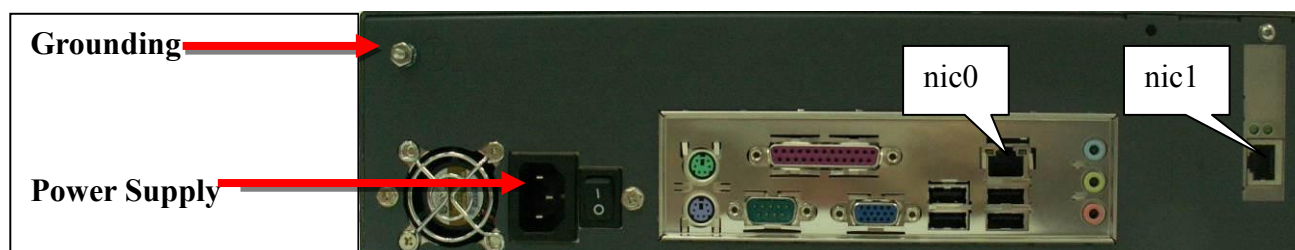
Figure 1: Grounding Screw on CXE2000 Rear Panel
