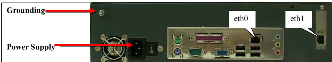
Figure 1: Grounding Screw on CXE2000 Rear Panel
