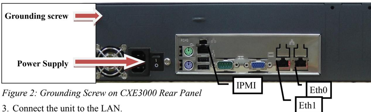
Figure 2: Grounding Screw on CXE3000 Rear Panel
