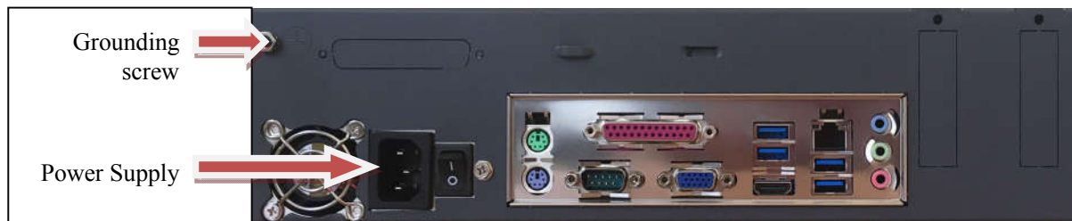
Figure 1: Grounding Screw on CXR2000 Rear Panel
