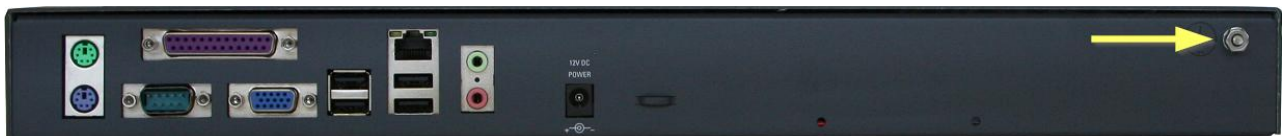
Figure 1: Grounding Screw on CXR1000 Rear Panel
