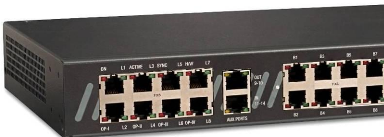
Figure 3: CXR1000 with 16 analog ports and I/O ports
