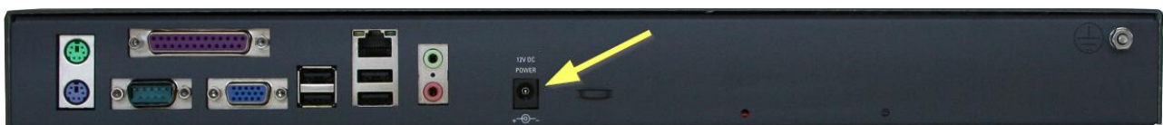
Figure 2: Power input socket on CXR1000 Rear Panel
