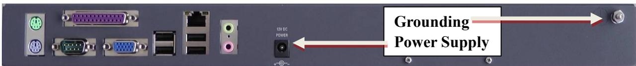
Figure 1: Grounding Screw on CXR1000 Rear Panel
