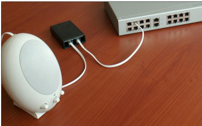
Figure 1: Rapid PA connected to Atribank and loudspeaker with internal amplifier
