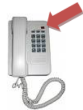
Figure 1: Typical analog phone with MWI neon light capability
