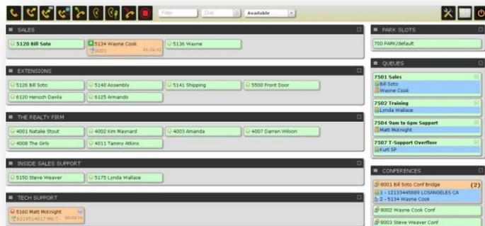
The enhanced switchboard (standard on CompletePBX CXE, CXT “Blue Steel” and CTS models; optional on CXR models) expands the functionality of the standard CXR version by supporting an unlimited number of active buttons (compared to 15), as well as providing instant messaging and voice mail explorer.
